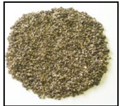
Very coarse sand makes for the best backfill.
