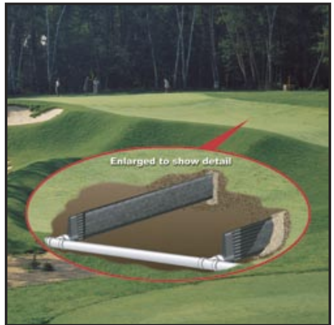
When an end or side outlet is used, the transport pipe is located at the same level as the bottom of the collectors.
