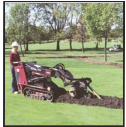
A walk behind trencher like this Toro is ideal. The 4-inch trench results in minimal disruption and minimal down time for the course.
