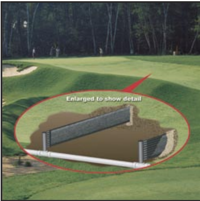
When a multi-purpose connector is used, the transport pipe is located beneath the level of the collector pipes.
